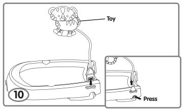
• Insert and "snap" the toy tab into either slot in the tray. *Hint:* To remove the toy, press the tab and lift the toy.
